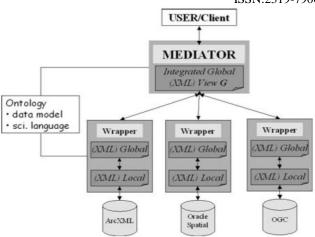
Figure 4. Extended Mediator Architecture [15]
