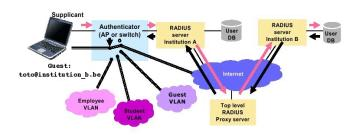
Fig. 2 Operational Mechanism of Eduroam
