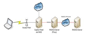
Fig. 3 RADIUS-based WiFi Roaming Authentication
