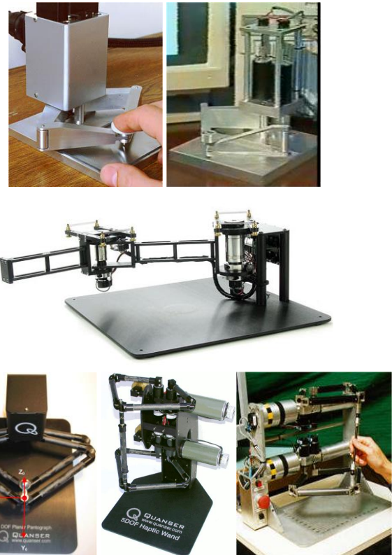
Figure 2. Images on the top line: Pantograph M1 [150], Pantograph medium [151]. Quanser Serial robot (in the middle) [154]. Images on the bottom line: Quanser 3DOF [106], Quanser 5DOF [107], Twin-Pantograph Haptic Pen [132].
