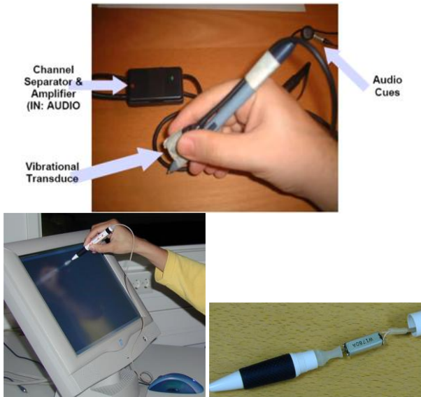
Figure 12. Vibrating pen AudioTact [142] (on the top) and Vibrating pen with a stopped rotor [158] (on the bottom).
