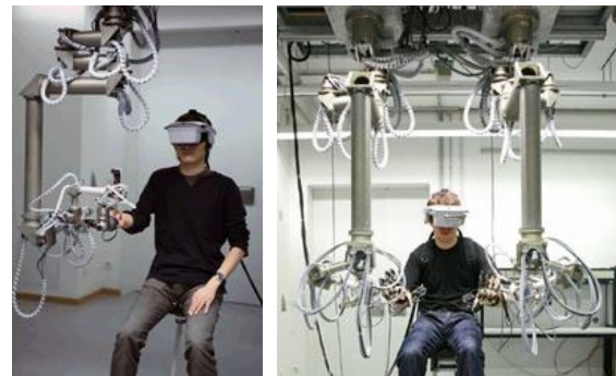
Figure 5. ViSHaRD10 - Virtual Scenario Haptic Rendering Device with 10 degrees of freedom offered a large workspace [138].
