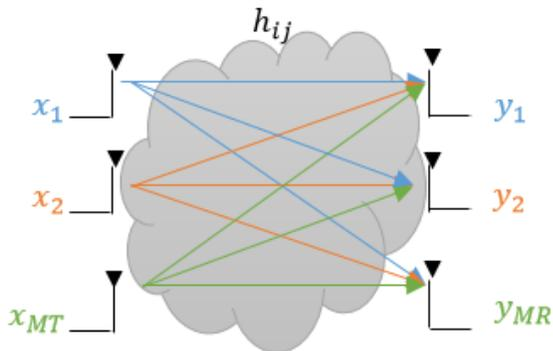
Figure 3: Illustration of MIMO Antennas
