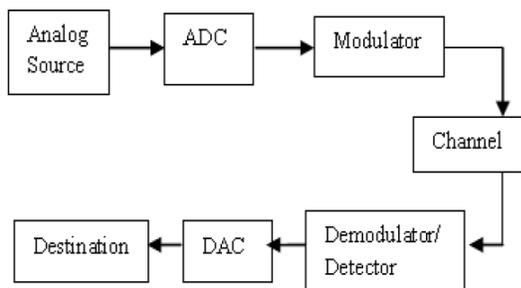
Figure 1: A typical digital communication system.
