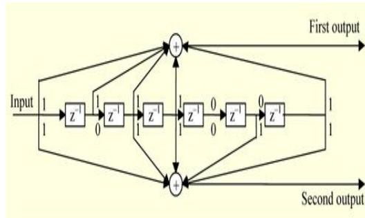
Figure 4: Convolutional Encoder Structure
