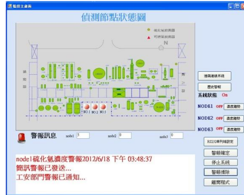
Figure 11. Sensor Node Status Display
