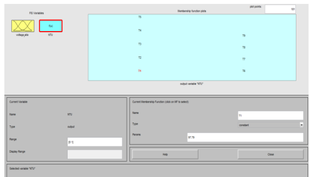
Fig8. membership function of the voltage ratio Fis turbidity model.
