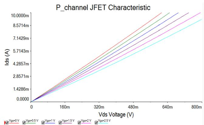
Figure 2. P-channel FET transistor characteristic
