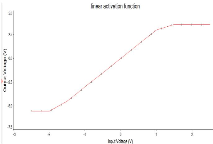
Figure 5. Response of the Activation Function
