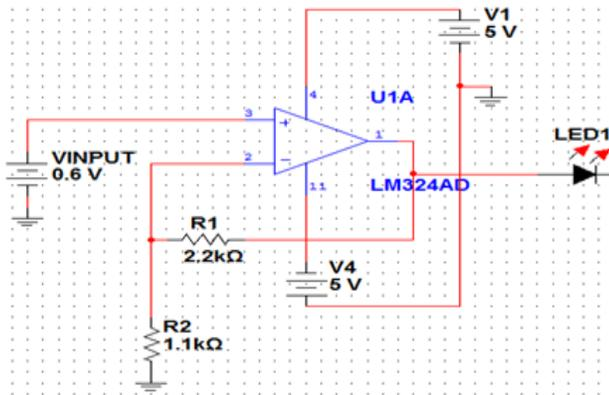
Figure 4. Schematic of Activation Function
