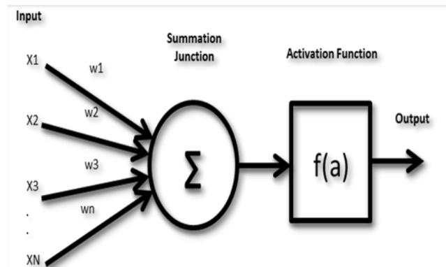
Figure 1. Structural Diagram of a Neuron
