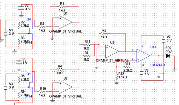
Figure 7. Logic AND Function
