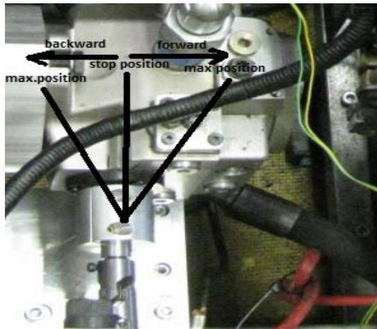
Figure 15 swash plate positions
