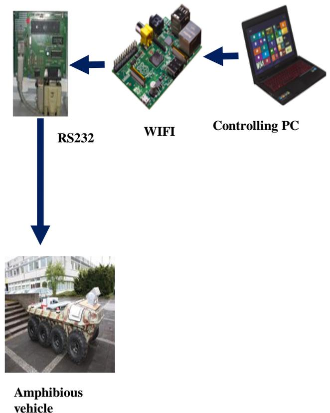
Figure 3 hardware structure of keyboard tele-operation
