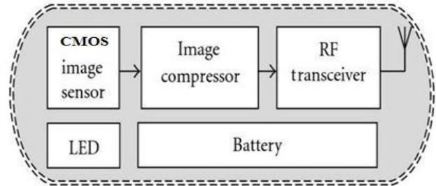
**FIG 6: Block diagram of a pill cam**
