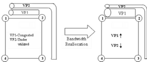
Fig. 1 Virtual path bandwidth reallocation.
