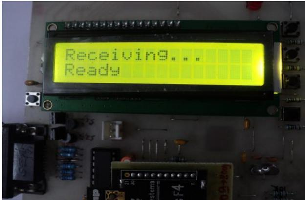
**Figure 9: Receiving status of data from PC to ARM**
