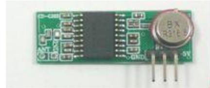
Figure 9: The RF Receiver Module
