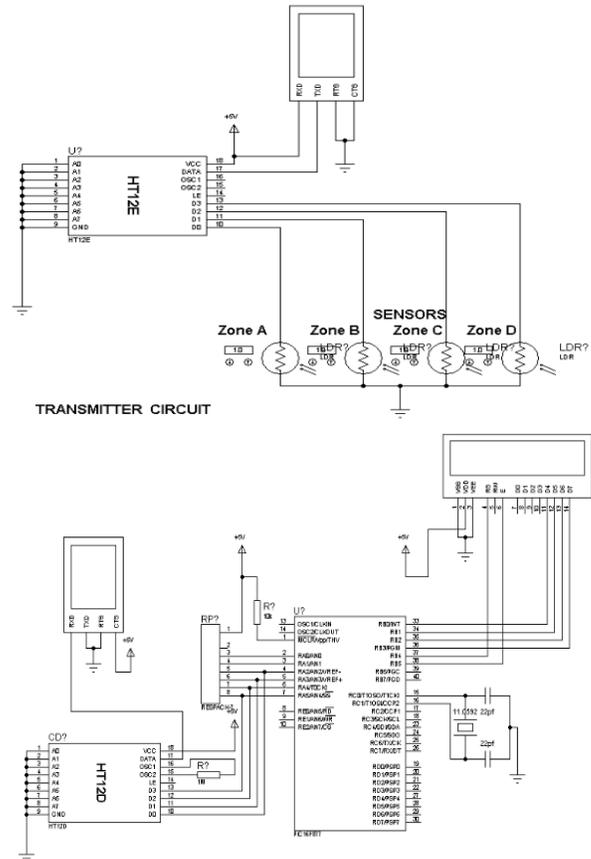
Figure 13: Receiver and Transmitter Circuits.
