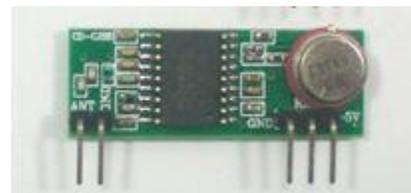
Figure 7: RF Transmitter Module
