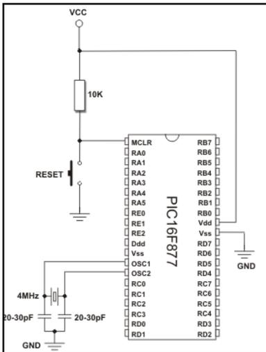
Figure 11: The basic connection of the PIC16F877A.
