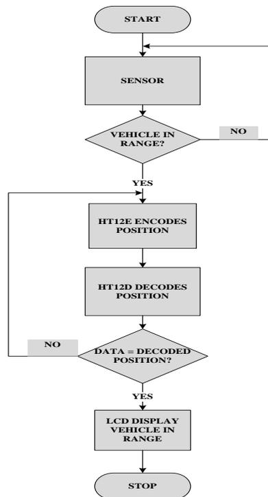
Figure 12: Flow Chart for System Design.
