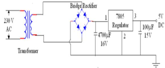
Figure 3: The Power Unit design Circuit.
