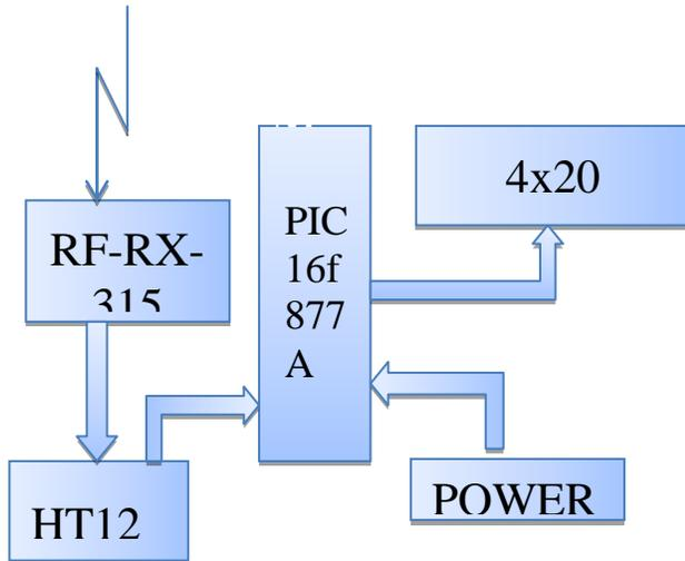
Figure 8: The interconnection of the Receiver unit.
