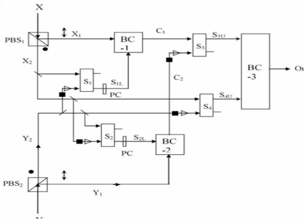
**Figure 2. All-optical quaternary QMIN(X, Y) circuit.** S: switch, NOLM: Non-linear optical loop mirror, PBS: polarizing beam splitter, BC: beam combiner, PC: polarization converter, EDFA: erbium doped fiber amplifier, WC: wavelength converter [12].
