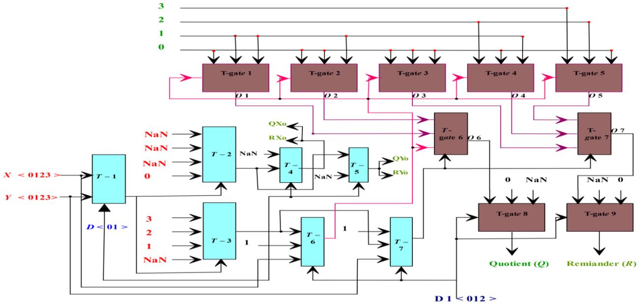
Fig.6. quaternary division operation with compact detect-zero circuit
