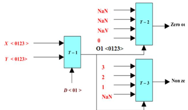
**Figure 5. Quaternary detect-zero circuit**
