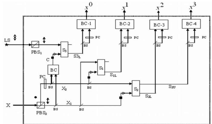
**Figure 3. All optical quaternary delta literal circuit [13].**
