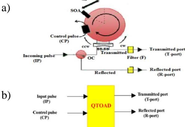
Figure 1. Terahertz optical asymmetric demultiplexer (TOAD) based switch. (a) Schematic diagram; CP: control pulse, SOA: semiconductor optical amplifier, OC: optical circulator, which
