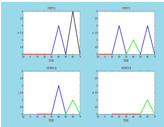
**Fig9. Simulated waveforms of quaternary division operation**
