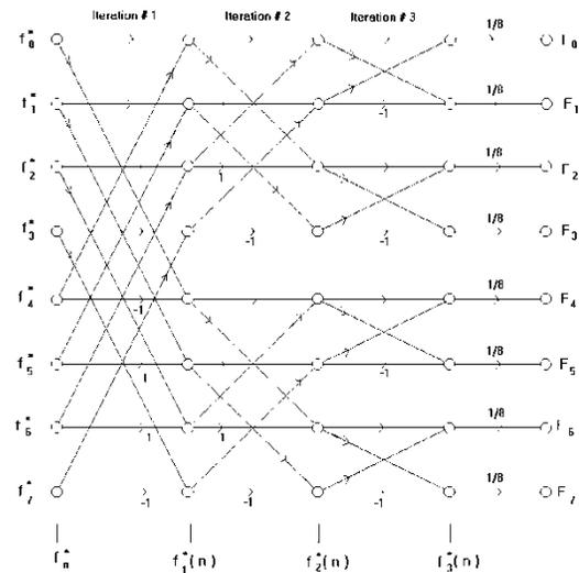
Figure 2. Signal flow graph of fast discrete Walsh transforms
