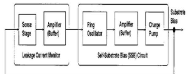
Fig 2. Elements of stabilization scheme.
