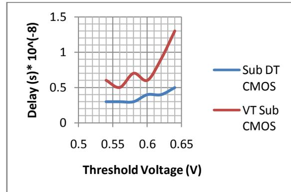
Fig 6. Delay Vs Threshold Voltage
