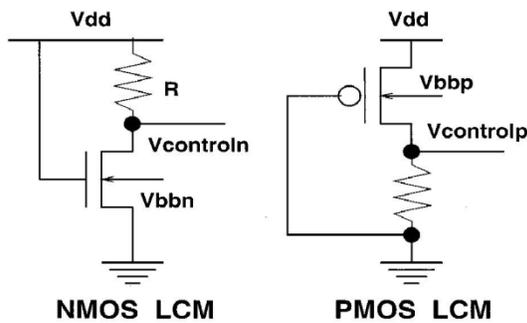
Fig. 3 Leakage Current monitors
