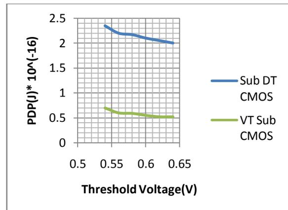
Fig 7. PDP Vs Threshold Voltage
