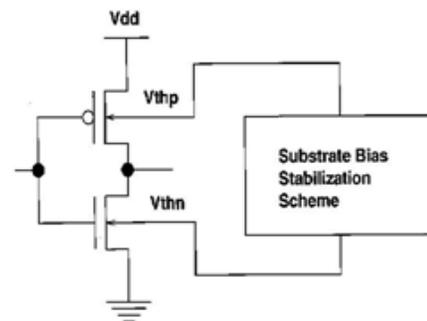
Fig.1 VT Sub CMOS Logic
