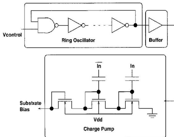
Fig. 4. Self-substrate bias circuit.
