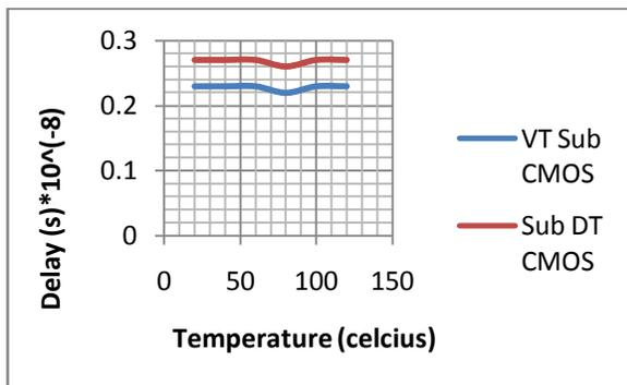
Fig. 4 Delay Vs temperature
