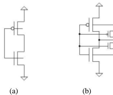
Fig 5. (a)Standard DT-CMOS
