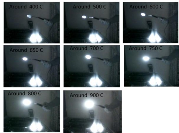
Figure (7) Heating steel piece in steps to obtain temperature – intensity relation
