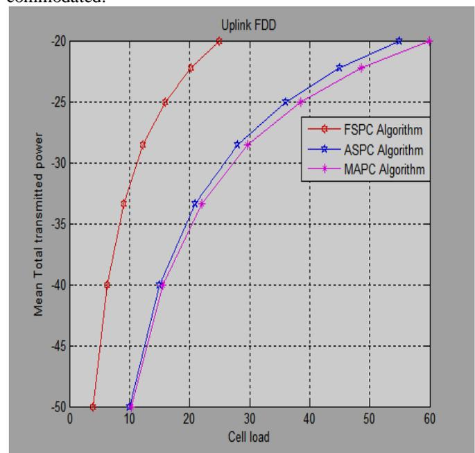
**Figure 2 Plot of the mean transmitted power as a function of the cell load for the various power control algorithms**
