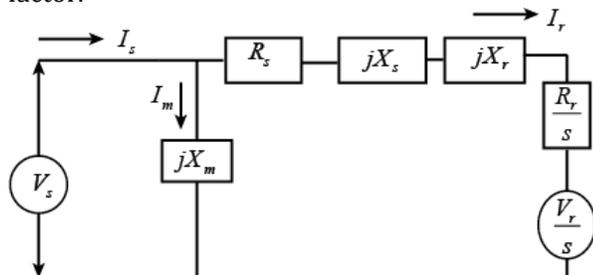
Figure 1(b) Equivalent approximated equivalent circuit of DFIAM with magnetizing branch transferred to stator [12].
