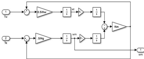
Fig. 5. Simulink model of Mechanical system
