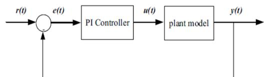
Fig. 2: A typical PI controls structure [13]
