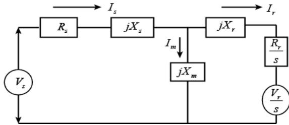
Figure 1(a) Equivalent Circuit of DFIAM with injected rotor voltage [12].
