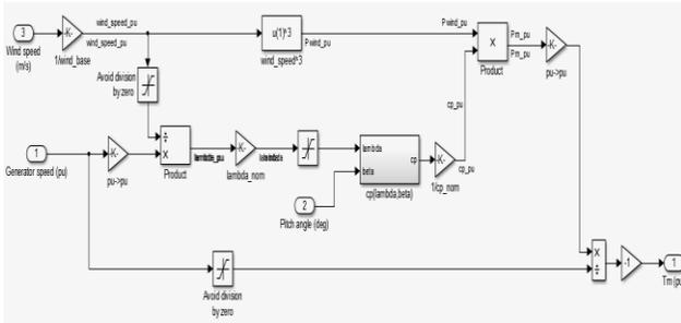
Fig.3 Simulation model of Wind turbine
