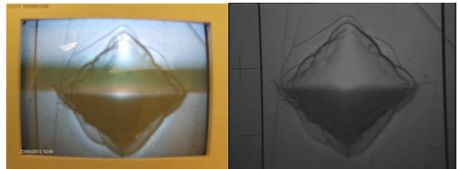
Figure 15. Left: Footprint captured by a commercial camera supplied by the manufacture of the microdurometer HM-124. Right: Footprint stored as JPG image by our image acquisition system.
