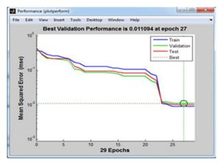
Fig. 5: The best performance plot of levenberg– Marquardt algorithm at 20 hidden layers
