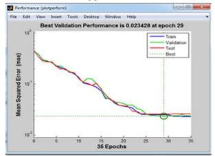
Fig. 6: The best performance plot of levenberg– Marquardt algorithm at 10 hidden layers
