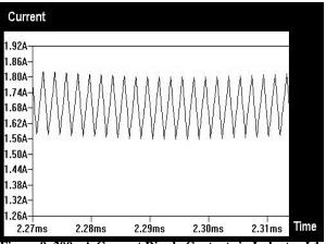
Figure 9. 200mA Current Ripple Contents in Inductor L1
