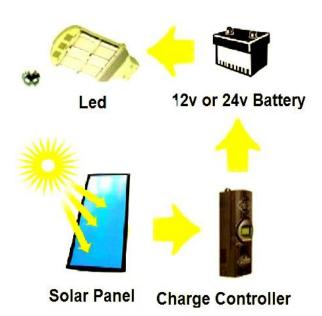
Figure 1. PV Street Lighting System with Charge Controller
