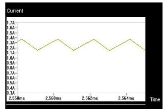
Figure 10. 200mA Current Ripple Contents in Inductor L2
