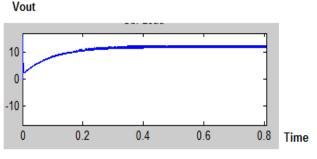
Figure 4. 12V output voltage of buck converter
