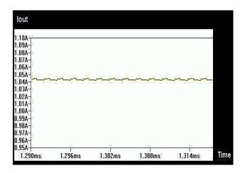
Figure 12. 1A Output Current of SEPIC Converter
