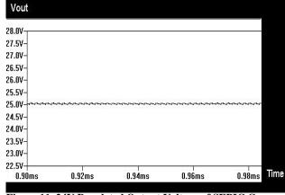
Figure 11. 24V Regulated Output Voltage of SEPIC Converter
