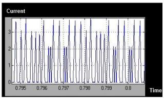
Figure3. Input Ripple Current of Buck Converter
