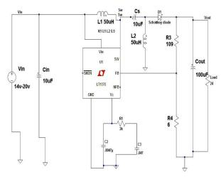
Figure 8. Simulated Circuit of SEPIC Converter in Ltspice Software
