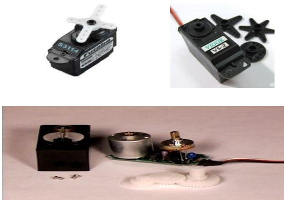
Fig.11: A Vigor Vs 2 and its parts
