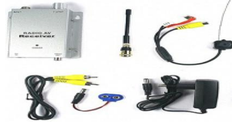
Fig. 16: Wireless camera and its accessories
