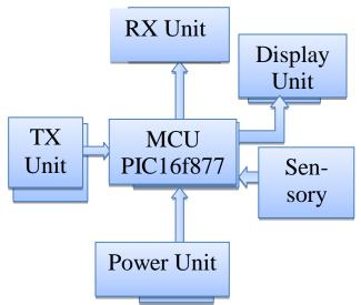
Figure 2: System Design Methodology
