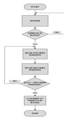
Figure 12: Flow Chart for System Design.
