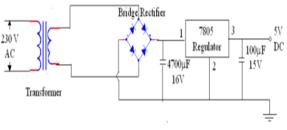
Figure 3: The Power Unit design Circuit.
