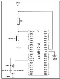
Figure 11: The basic connection of the PIC16F877A.
