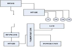
Figure 5: Interconnection of LDR and other Circuitry.
