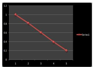
Figure 14: Graph of resistance of LDR versus Light intensity in Table 1.
