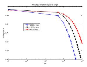
Figure 6. Throughput for different fixed packet lengths
