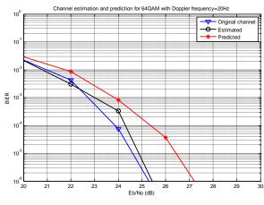
Figure 2. performance for  $64QAM f_d = 20Hz$
