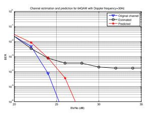
Figure 3. performance for  $64QAM f_d = 30Hz$
