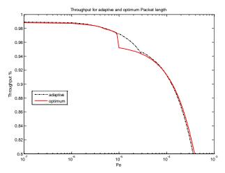
Figure 7. Throughput versus channel probability of error
