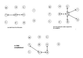
Figure 2.1. Resolving failed link in DSDV
