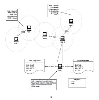
Figure 3.1.: Working of AODV routing protocol
