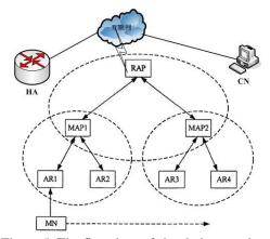
Figure 5. The flowchart of simulation topology During the simulation process, MN moves as description at VI, wherein the AR1-AR2 movement is anchor domain
