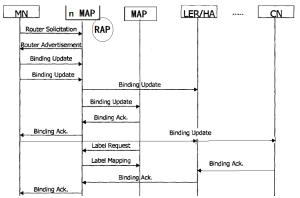
Figure 4. The switching process in the same RAP domain for MN
