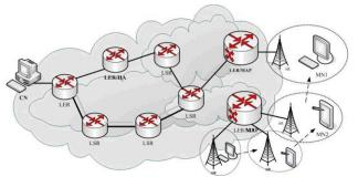
Figure 3. MPLS based HMIPv6 access hierarchical network
