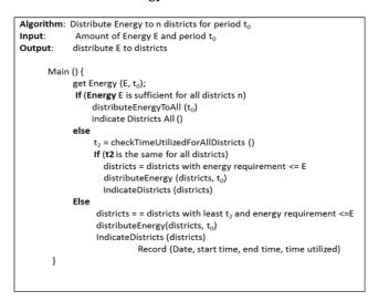
Figure 1. Electricity Distribution Algorithm
