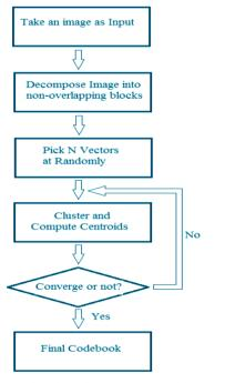
Figure 1: The flowchart of LBG clustering algorithm
