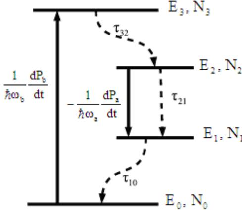
Figure 1. Four-level atomic systems model.
